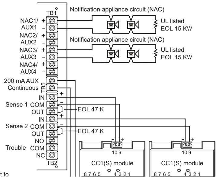
\*The Booster supports AC Power fail delay of three hours via its trouble contact when dip switch SW2-6 is on. All other troubles are reported to supervising module or panel without delay via Sense inputs.
